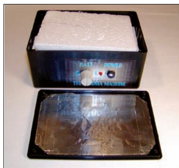
Figure 5. The last piece of foam is in place. The high voltage wire goes over the top of the foam and presses against the foil inside the plastic cover.
