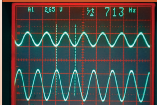
Figure 15. This photo says it all. The top sine wave's amplitude decreased as I increased the input frequency towards the digital filter's 1 kHz bandstop value.
