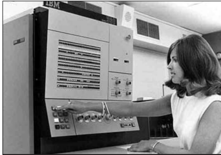
The System/360 Model 22 was introduced as a general purpose computer that combined intermediate-scale data processing capability with small system economy. Its main storage was either 24K or 32K. Photo courtesy of International Business Machines Corporation . Unauthorized use not permitted.
