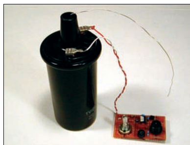
Figure 3. Completed electronic assembly. The PCB mounts to the plastic case and the power jack.
